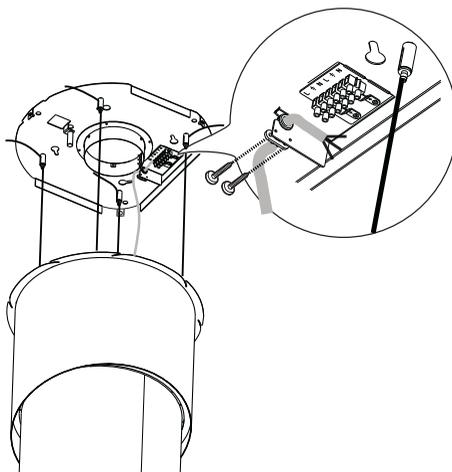
Finally, check that the power supply cable is properly locked, checking that when the mobile unit rises up towards the ceiling, it positions itself over the mobile unit and does not come out from the edge of the hood.
