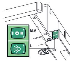
**L** Light Switches the lighting system on and off.
