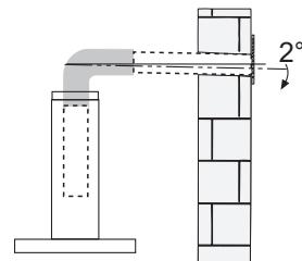
When the cooker hood is used in conjunction with appliances supplied with energy other than electric, the negative pressure in the room must not exceed 0,04 mbar to prevent fumes being drawn back into the room by the cooker hood.
